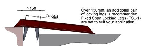
Over 150mm there is a significant risk of the board separating from vehicle - this is <u>not recommended</u>.
